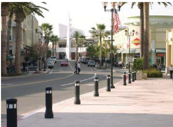
Access in high activity areas can be controlled through traffic circles, signage, bollards and striping.
